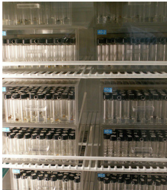
Fig. 1 Minimal growth preservation of living plant cells in a Plant Growth Incubator at 10°C and 10-15 µmol m -2 s -1 PPF by fluorescent lamps with 12 h photoperiod.
