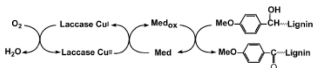
Fig. 3 The oxidation cycle of a laccase/mediator system towards non-phenolic substrates. (Figure re-printed from Astolfi et al. (2005) New Journal of Chemistry , 29, 1308-1317, with kind permission of the Royal Society of Chemistry).
