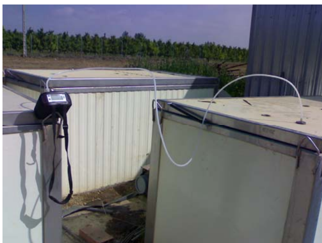
Fig. 7 Gases measurement system inside the composter by an automatic analyser.
