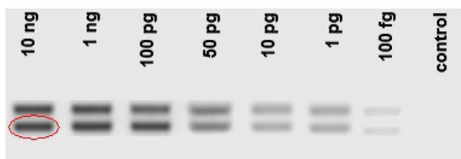
**Fig. 4** Sensitivity of LightCycler PCR assessed by using 7-fold dilutions of *F. solani* DNA. Primer pair's ITS-Fs8 generated distinct amplified fragments up to 100 fg. Negative controls with no DNA (control).
