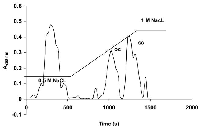
**Fig. 4** Adsorption of the pDNA from unclarified lysate by expanded bed technique on streamline DEAE as adsorbent (column with 13 mm in diameter).
