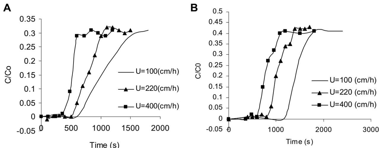
**Fig. 3** Nanobioparticle breakthrough curves in the expanded bed of the streamline DEAE adsorbent. (A) BSA nanoparticle BTCs. (B) plasmid DNA nanoparticle BTCs.
