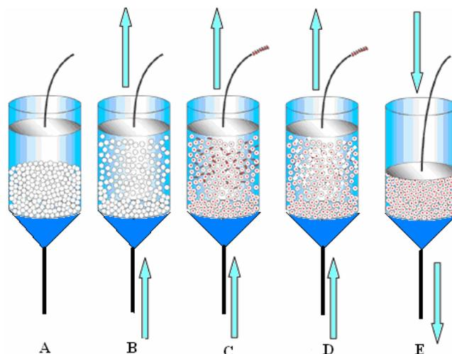
**Fig. 2** Operating procedure of expanded bed adsorption. Details of A-E in text.
