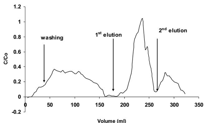
Fig. 6 Expanded bed recovery of BSA nanoparticle with streamline DEAE in column with 1.3 cm in diameter.
