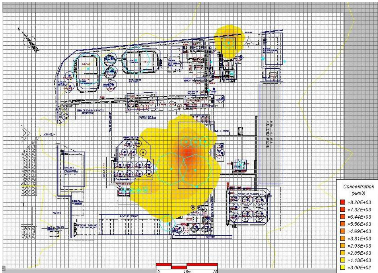
Fig. 1 Example of dispersion modelling output: odour concentration mapping at an industrial facility.
