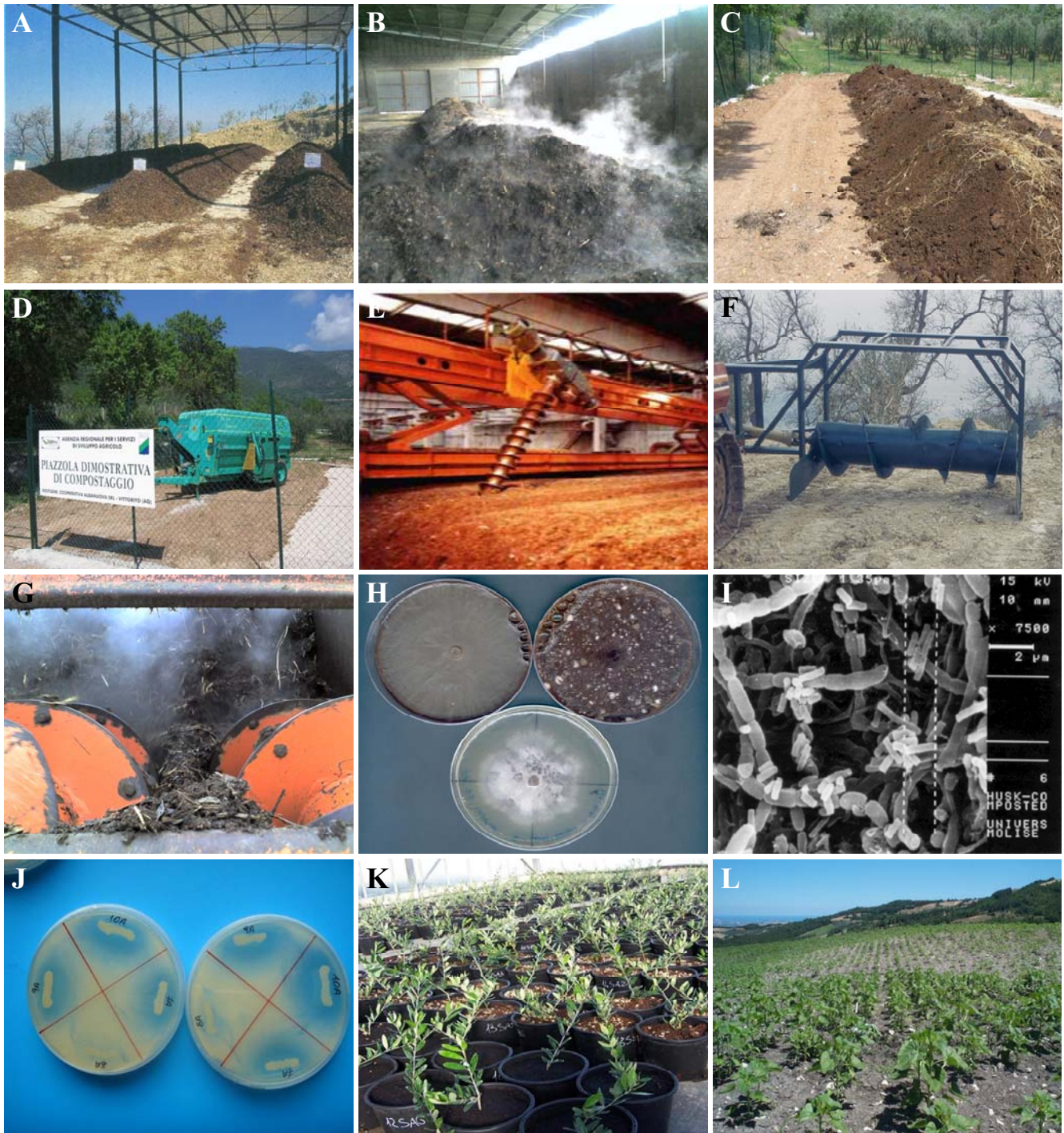
Fig. 2 Images of composting processes carried out in the last decade. (A) Composting process carried out on 2-POH in pilot scale plant. (B) 2-POH composting carried out in confined pilot scale plant. (C) Composting of 3-POH carried out in open air pilot scale plant. (D) Composting pilot plant and turning/grinding machine. (E) OH composting carried out in industrial scale plant. (F) Prototype of the turning machine realized. (G) Olive mill and agricultural residues turning and grinding. (H) In vitro suppressive test on Verticillium dahliae . (I) SEM observation (7500 x) of a sample of composted OH. (J) In vitro activity of antagonistic bacteria isolated from compost. (K) In vivo suppressive trials carried out in a nursery on young olive plants. (L) Agronomical trials carried out in open field on sunflower.
