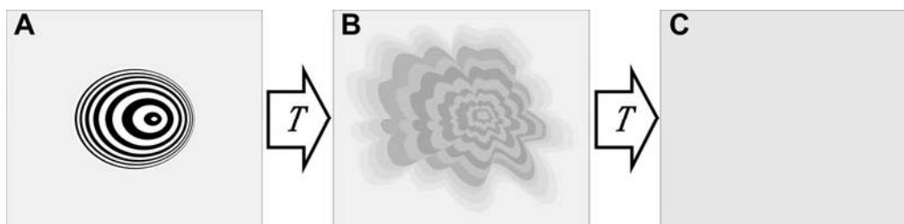
Fig. 1 Schematic diagram of heat gelatinization of a starch granule (A) Starch granule suspended in water: cross section of the granule presents lamellar structure of concentric ellipsoids. (B) Heating induces the swelling and disruption of the granule. Molecular motion is accelerated by heating and the lamellar structure is lost by swelling. (C) Further heating leads to the complete gelatinization where the granular shape is not observed. (A-C) Figures re-printed from Yamamoto K, Fukami K, Kawai K, Koseki S (2006) (Pressure gelatinization of starch). Food and Packaging (Shokuhintoyouki) 47, 448-456, with kind permission from the Institute of Canning Technology, ©2006.
