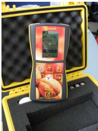
Fig. 4 The DA-Meter portable instrument. The dimensions of the instrument are 15 cm by 8 by 5 (length, width, thickness).
