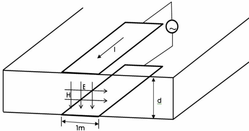
Fig. 5 Fields between conductors of a line strip.
