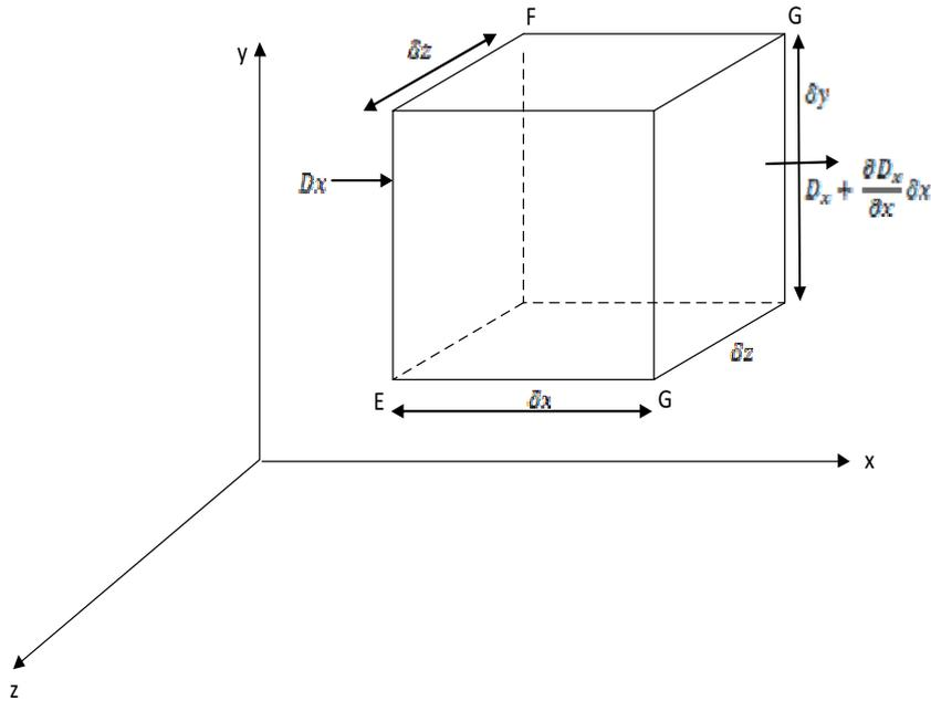
**Fig. 1 Divergence of electric flux density.** The positive X-direction shows an increase in the electric flux density
