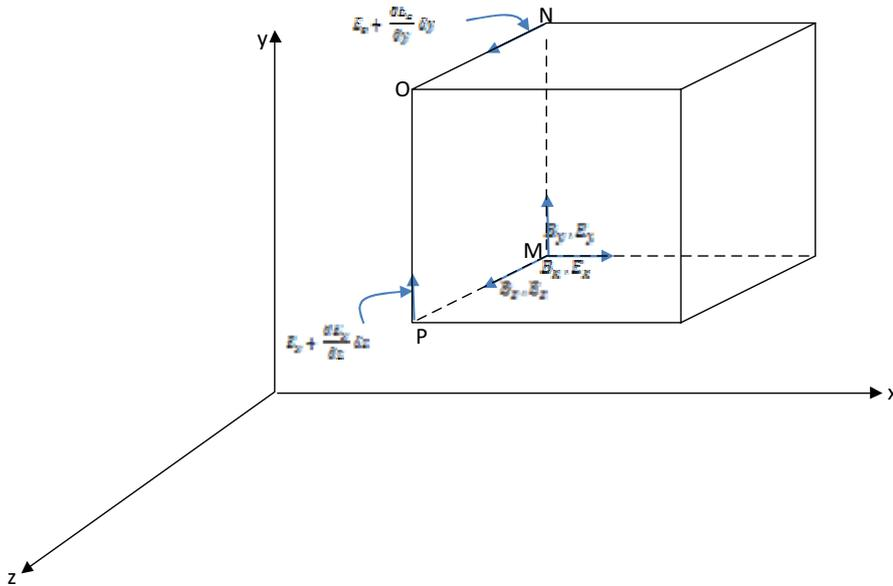
**Fig. 3 Alternating electric and magnetic fields in space.** The above diagram shows a general representation of magnetic field and electric field components as well as electric fields component increases along the Y- and Z-axes, respectively.
