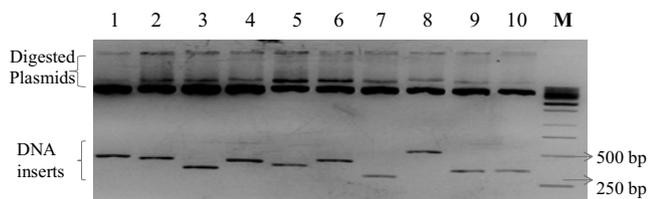
Fig. 6 Restriction digestion of cloned plasmids with *EcoRI*. Lane M: 1-kb marker, Lanes 1-10: Digested plasmids with inserts.
