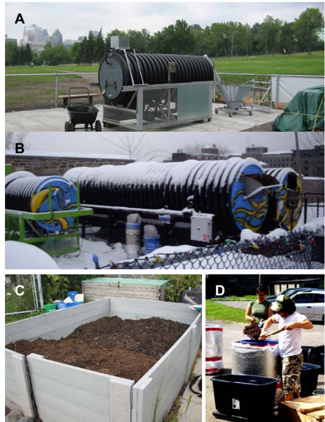
Fig. 1 The experimental 1.4 m 3 composter built of double polyethylene tubing with a corrugated exterior wall (A) aerated by turning at 5 rpm and by leaving the top door open otherwise; the 2 larger reactors added in 2005 and 2009 besides the smaller prototype on the left (B). The compost maturation box for the Tournesol Community Composting Centre built of wood slates (C). Barrels used as experimental laboratory composters for the active phase (covered with an aluminum water-proof liner insulated blanket) and containers used for the maturation phase (rectangular container) (D).
