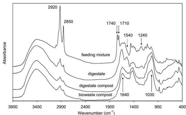
**Fig. 4** Changing spectral characteristics during anaerobic (wet process) and aerobic degradation.
