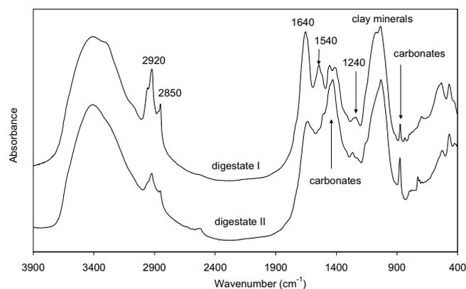
**Fig. 2** Infrared spectra of digestates from wet (I) and dry (II) anaerobic processes.
