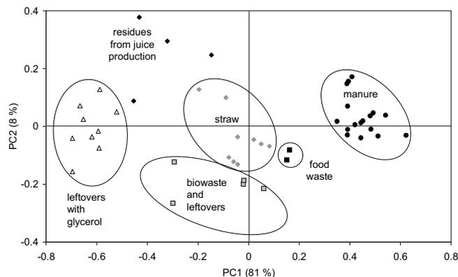
**Fig. 3** Principal component analysis of digestates from different input materials and similar wet digestion processes, based on infrared spectra (wavenumber range from 4000–400  $\text{cm}^{-1}$ ).
