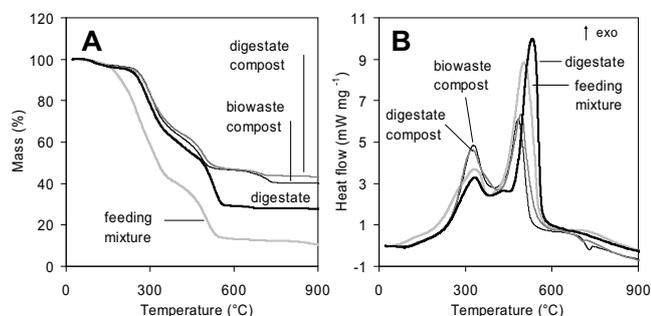
**Fig. 5** Changing thermal characteristics during anaerobic and aerobic degradation. (A) Mass losses (thermogravimetry), (B) heat flow profiles (differential scanning calorimetry).
