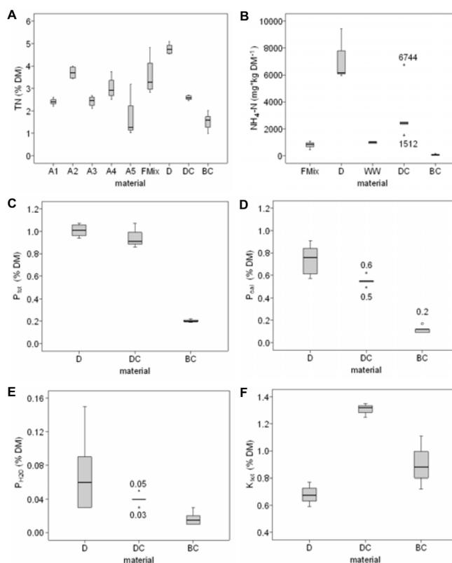
**Fig. 6** Minima, maxima, median, 25% and 75% quantile of total (A) nitrogen (TN), (B) NH<sub>4</sub>-N, (C) total phosphorus (P<sub>tot</sub>), (D, E) extractable phosphorus (CAL and H<sub>2</sub>O) and (F) total potassium in input materials (A1 – A5), feeding mixtures (FMix), digestates (D), waste water (WW), composted digestates (DC) and biowaste compost (BC).
