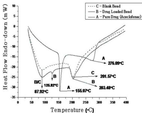
Fig. 2 DSC curve for pure drug, drug loaded bead and blank bead.
