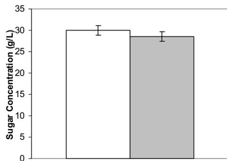
Fig. 1 Sugars present in acid hydrolysate before (white bar) and after (grey bar) detoxification. n = 3. Bar = SEM
