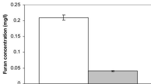
Fig. 3 Furans present in acid hydrolysate before (white bar) and after (grey bar) detoxification. n = 3. Bar = SEM
