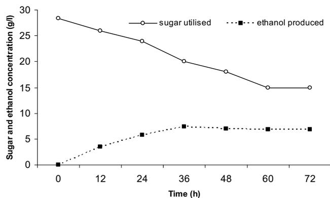
Fig. 5 Ethanol production by monoculture of *S. cerevisiae* VS3 at 30°C, using *Sorghum straw* acid hydrolysate. n = 3. Bar = SEM
