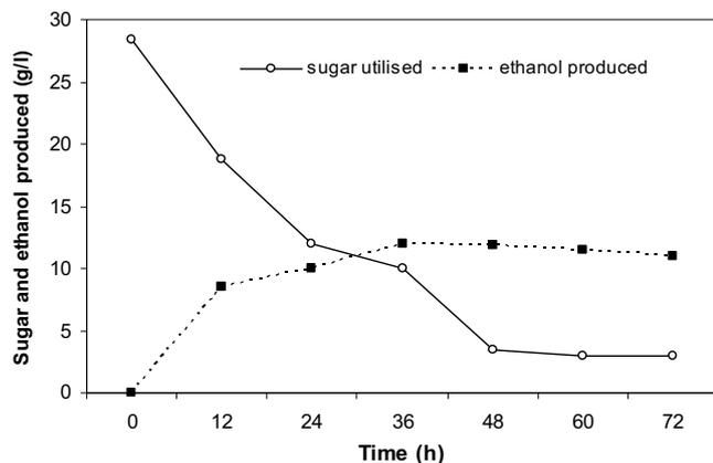
**Fig. 6** Ethanol production by co-culture of *P. stipitis* NCIM 3498 and *S. cerevisiae* VS3 at 30°C, using *Sorghum bicolor* acid hydrolysate. n = 3. Bar = SEM
