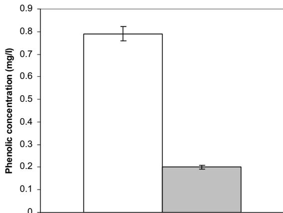
Fig. 2 Phenolics present in acid hydrolysate before (white bar) and after (grey bar) detoxification. n = 3. Bar = SEM
