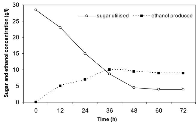
Fig. 4 Ethanol production by monoculture of *P. stipitis* NCIM3498 at 30°C, using *Sorghum straw* acid hydrolysate. n = 3. Bar = SEM
