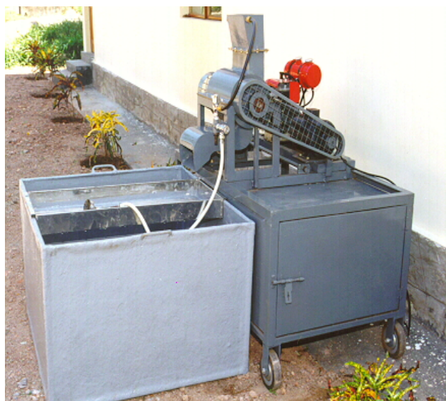
Fig. 1 Multipurpose mobile starch extraction plant for sweet potato starch extraction.
